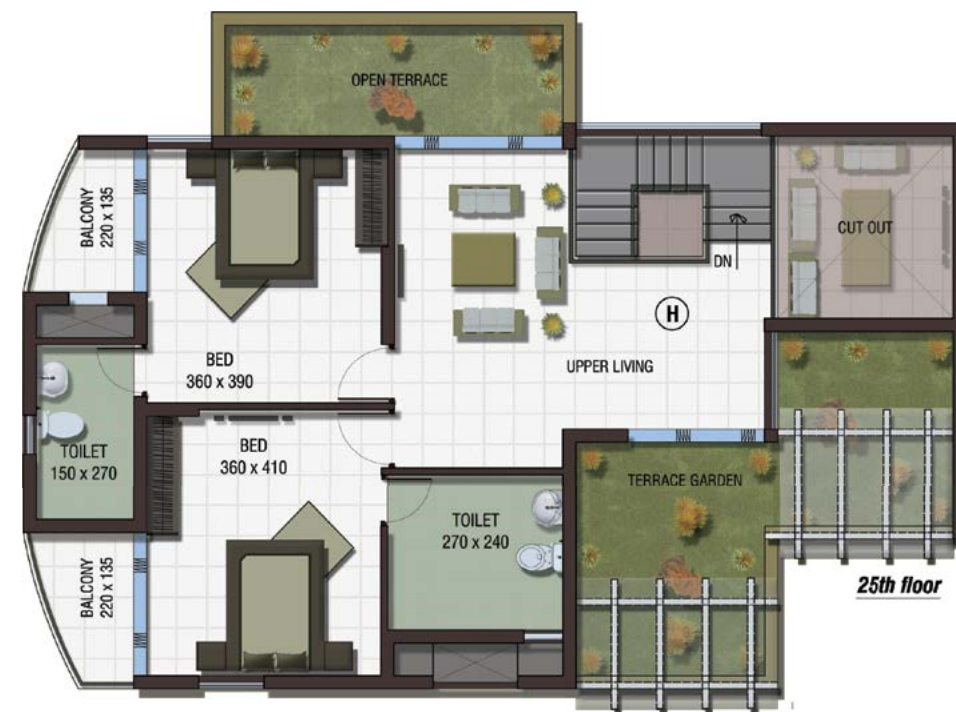
Type H - 4BHK Area-2988+425 sq. ft Not to Scale. All dimensions are in Cm.
