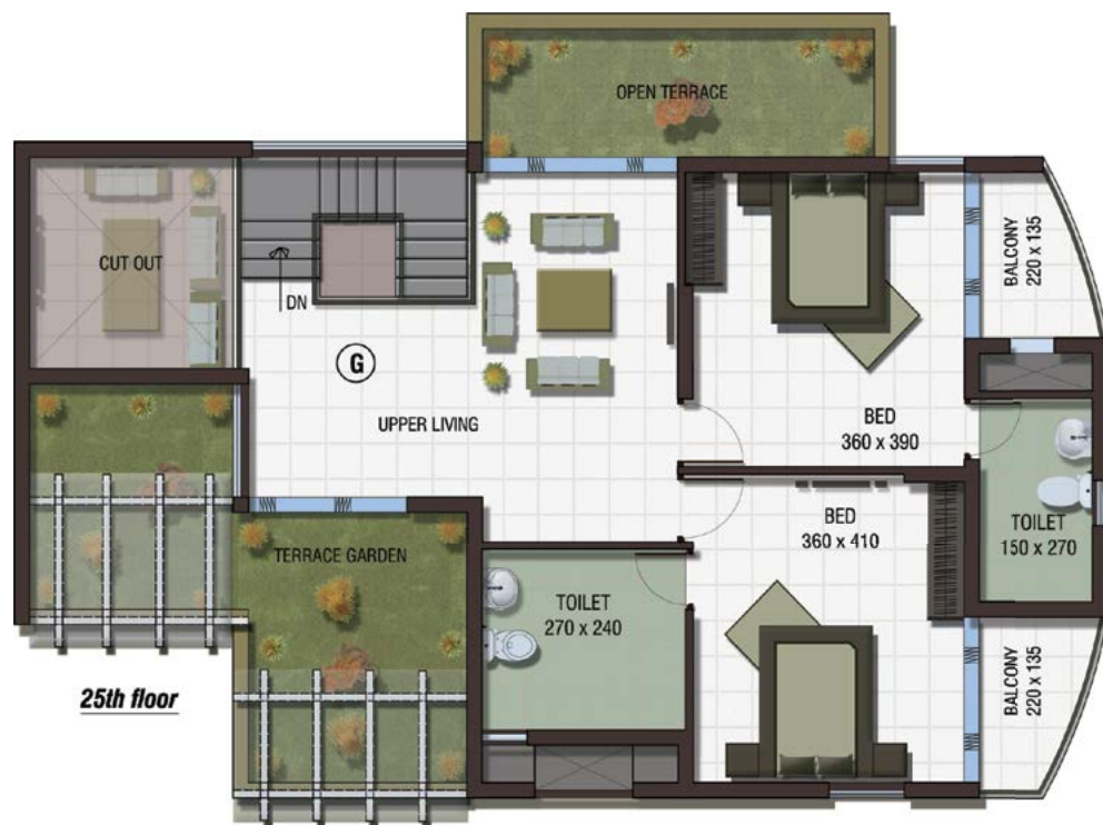
Type G - 4BHK Area-2983+425 sq. ft Not to Scale. All dimensions are in Cm.
