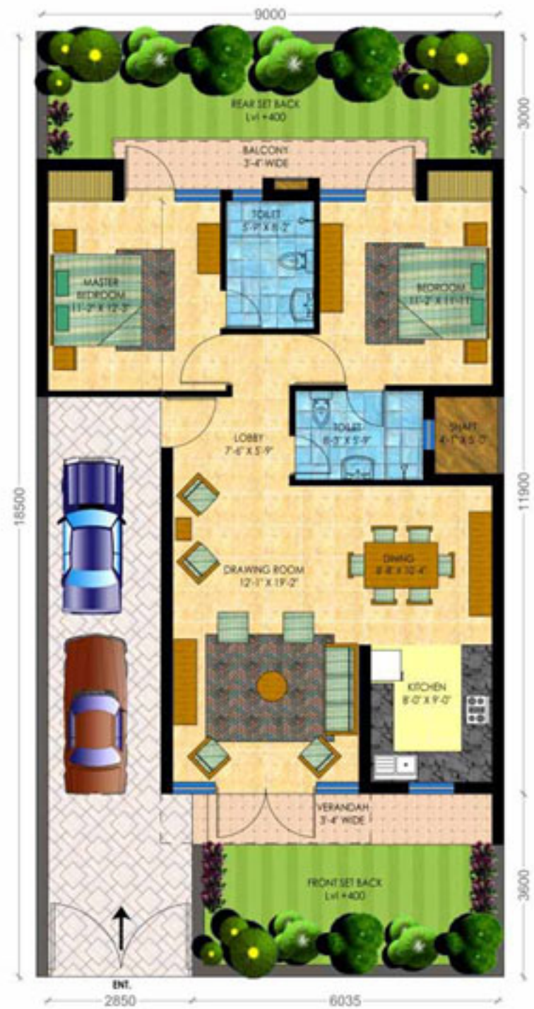
GROUND FLOOR PLAN ON 200 SQ.YDS. PLOT ( 9.00 X 18.50 M.) SUPER BUILTUP AREA - 1150.00 SQ.FT.
