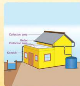
Rain Water Harvesting
