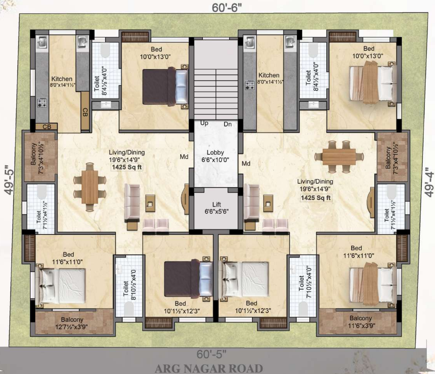
TYPICAL FLOOR PLANS (1st - 3rd floor)
