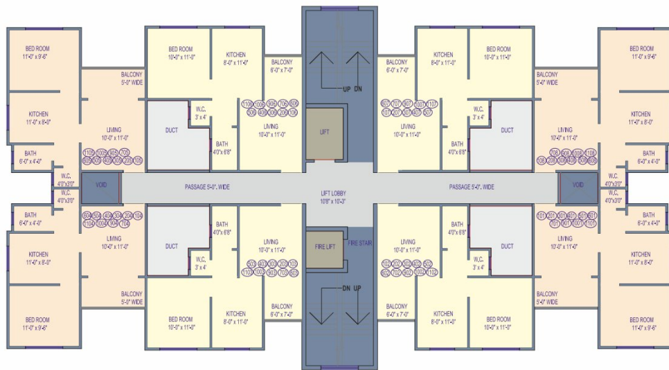
TYPICAL 1st to 7th & 9th to 11th FLOOR PLAN Building 3
