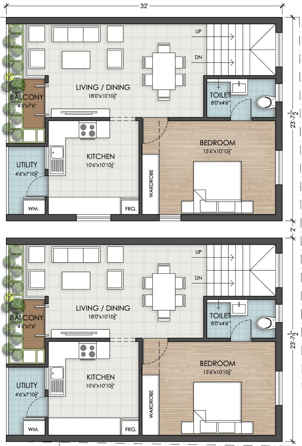
FIRST FLOOR PLAN BUILDING - 756 SQ.FT.
