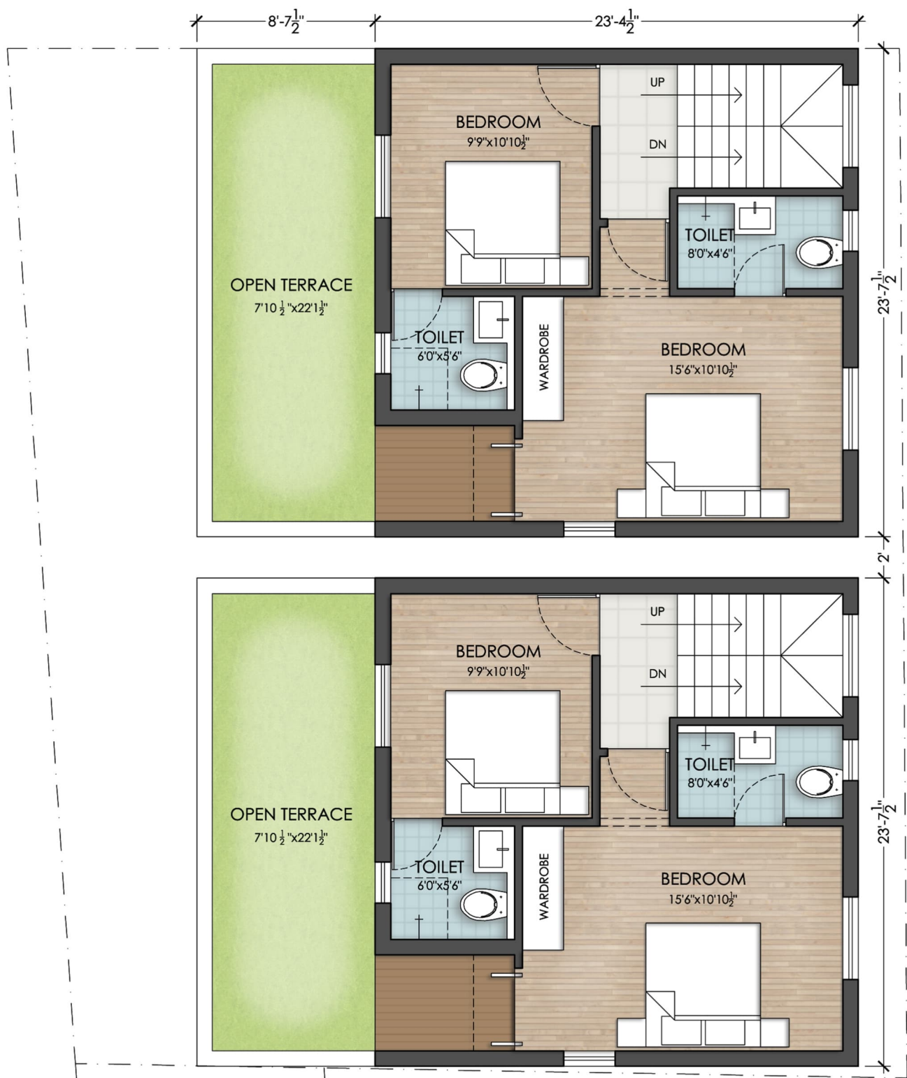
SECOND FLOOR PLAN BUILDING - 552 SQ.FT.
