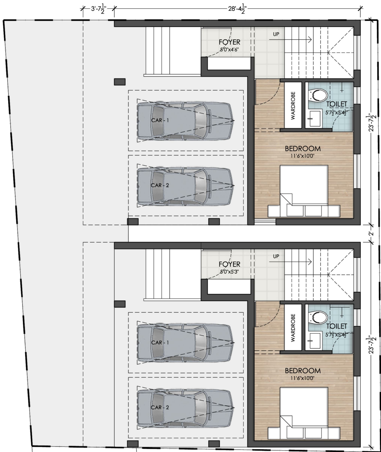
STILT CUM GROUND FLOOR PLAN BUILDING - 343 SQ.FT. STILT - 327 SQ.FT.
