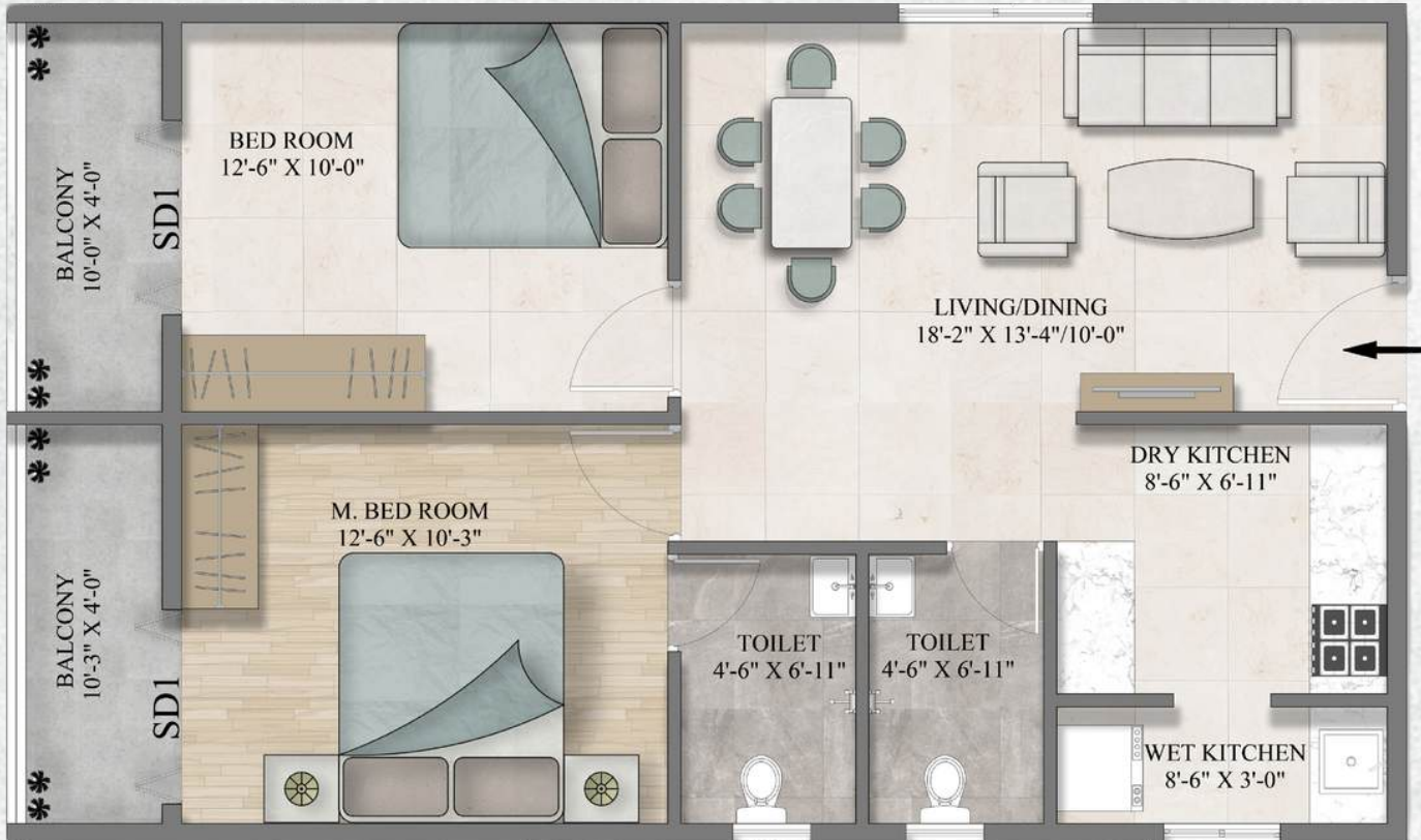
Typical Floor | 2 BHK | 1040 Sft | East Facing Unit Number - 04,05,06,07,08,09,10,11,12 (Block B)
