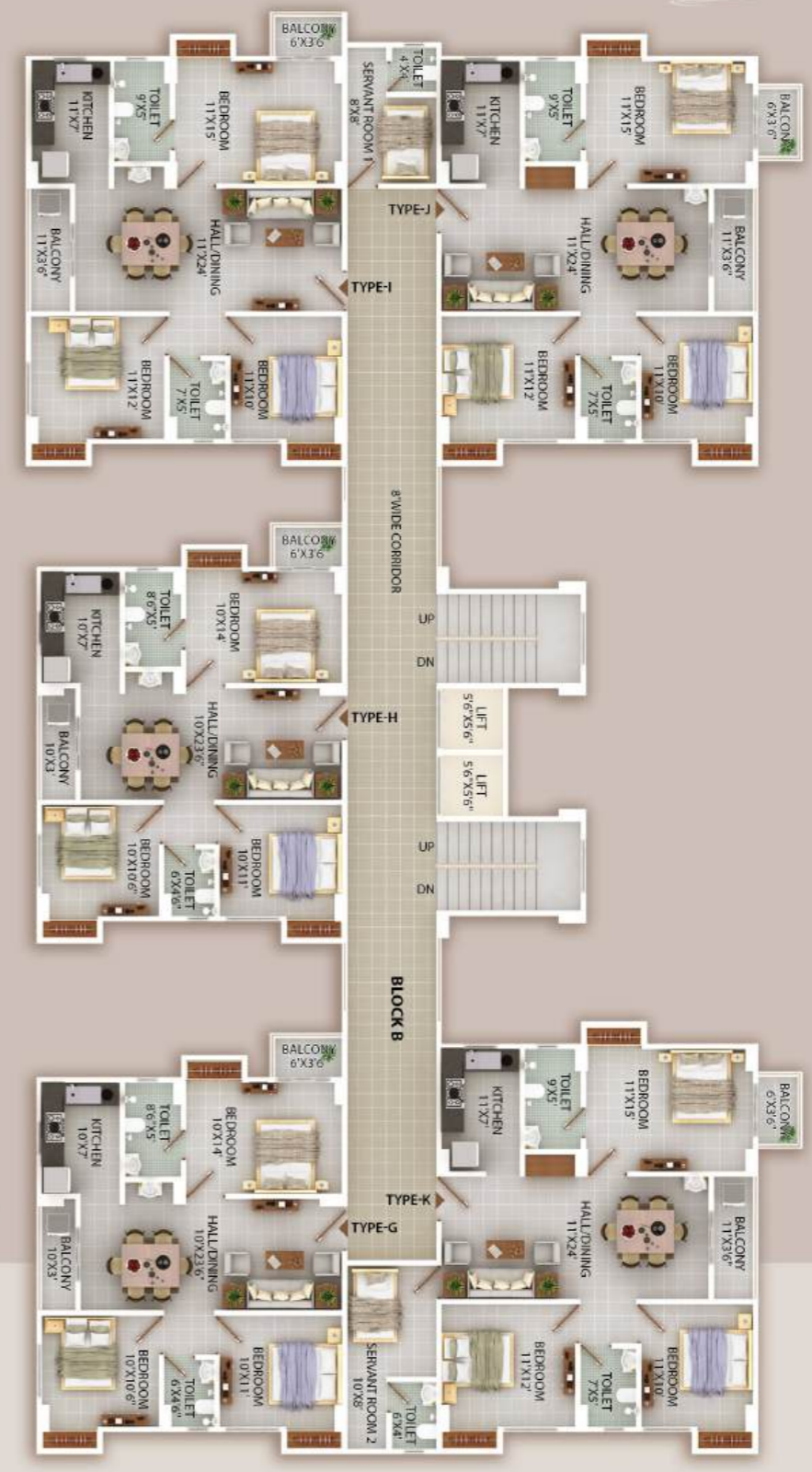
BLOCK B 1ST TO 10TH TYPICAL FLOOR
