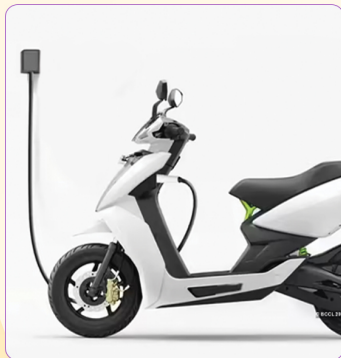
Two Wheeler EV Charging Point
