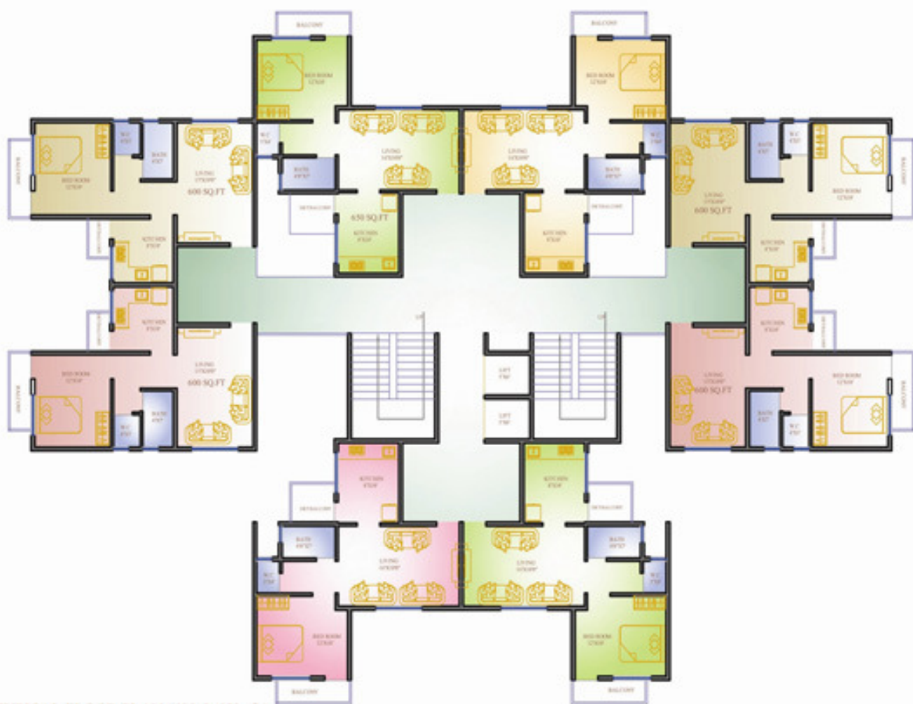
TYPICAL FLOOR PLAN (600 & 650 sft.)
