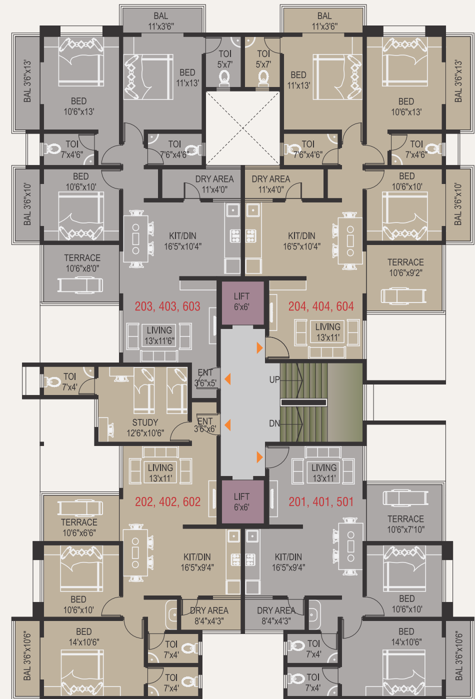
TYPICAL 2nd,4th,6th FLOOR PLAN
