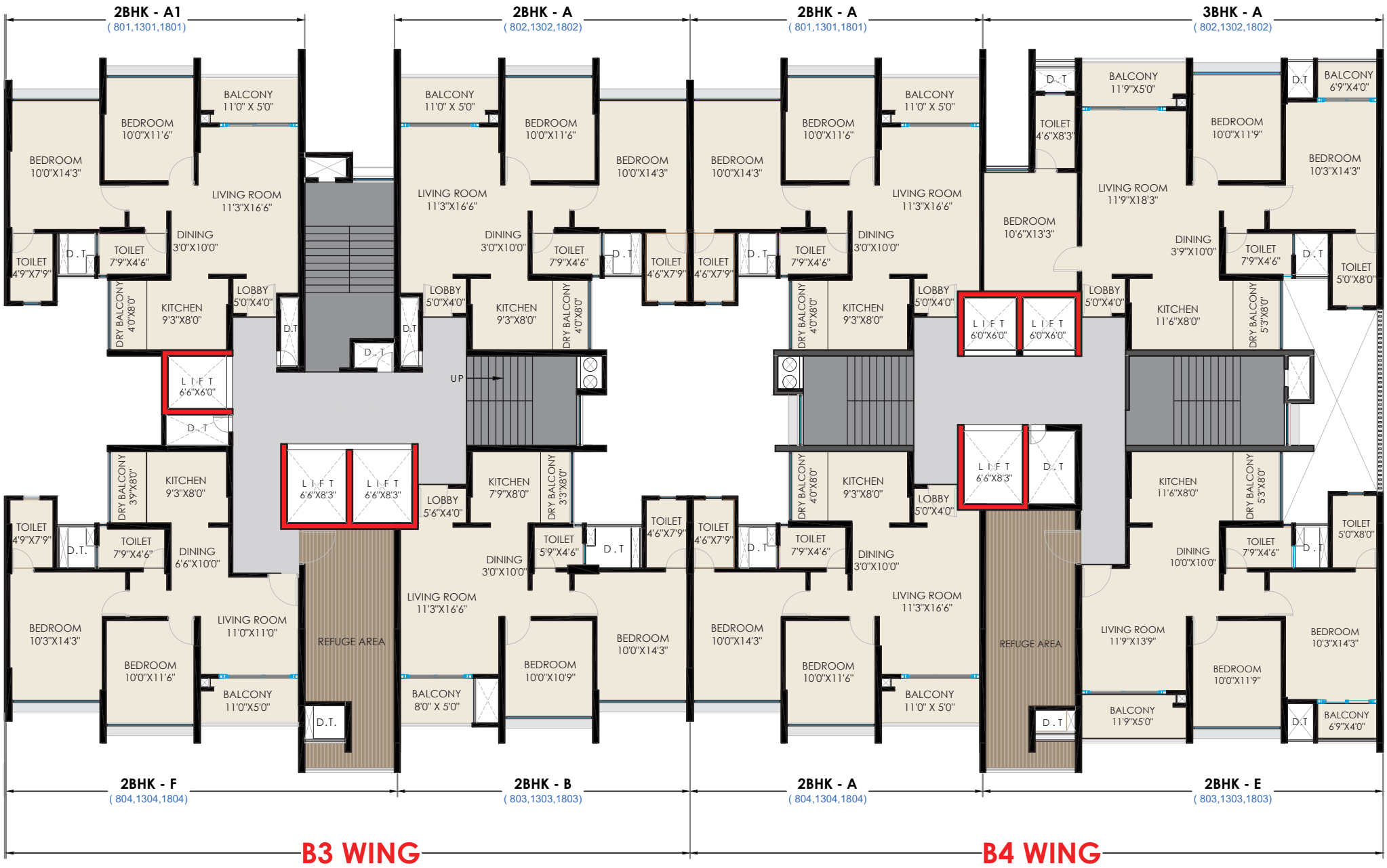
REFUGE FLOOR - BUILDING B
